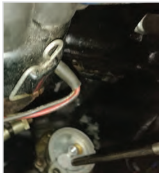
Cleaning the Fuel Pump with compressed air.
