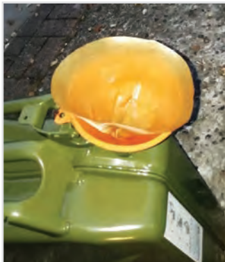
Using a paper coffee filter paper in a funnel to clean the sediment of the fuel.
