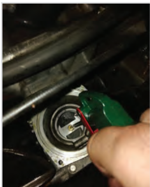
Blowing through the main jet from above with compressed air with the Carburettor Top, and piston/needle assembly removed.
